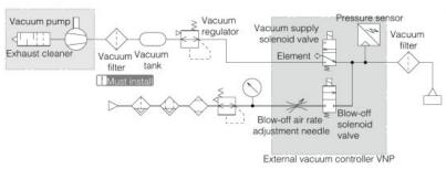
Compressed air is not necessary for suction transport by using the external vacuum controller VNP, which have direct operating valve for vacuum supply and blow-off solenoid valve. (Compressed air is necessary for blow-off.) Therefore, the consumption amount of compressed air can be remarkably reduced
